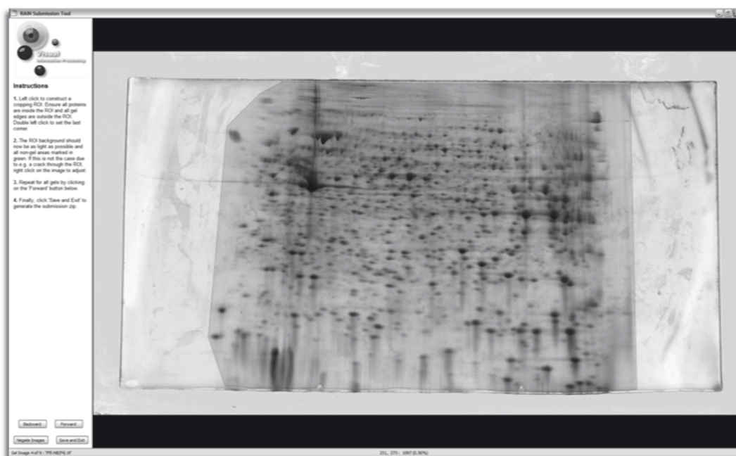
Fig. 1. Gel image cropping with the RAIN submission tool. The shaded area shows an optimum polygonal crop that removes the gel edges and some artifacts while retaining the protein spots
